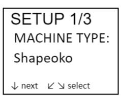
By turning the Knob, the type of the machine used for controlling may be selected. This setting only determines what states at the enable inputs are required for controlling the laser.
