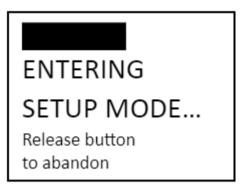
Hold the Button for at least 3 seconds, until the progress bar is filled. Otherwise, the SETUP mode will be skipped and the CNC Adapter will enter the DISARMED mode.
