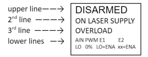
The upper line displays the name of the current working mode.
