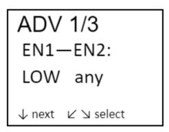
Here, the option of the enable inputs may be changed manually. This option specifies the necessary states for the ENABLE 1 and ENABLE 2 inputs to allow the input signals to enable the laser.
